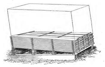
Fig. 81.—Lumber piled lengthwise on wooden foundation.
